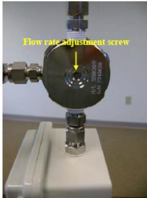
Figure 4. Flow rate adjustment screw
