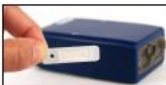
Figure 7: White sample deposit side of filter strip faces the top.
