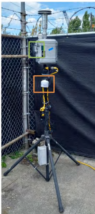
Figure G-1: illustration of the N-FRM installation at our UEWA (Fontanelle St.) site, with Purple Air sensor added to the setup(left). The other two photos (borrowed from Purple Air© and ARA instruments© websites), provide a more detailed look at the N-FRM RTP (upper right) and Purple Air sensor (lower right).
