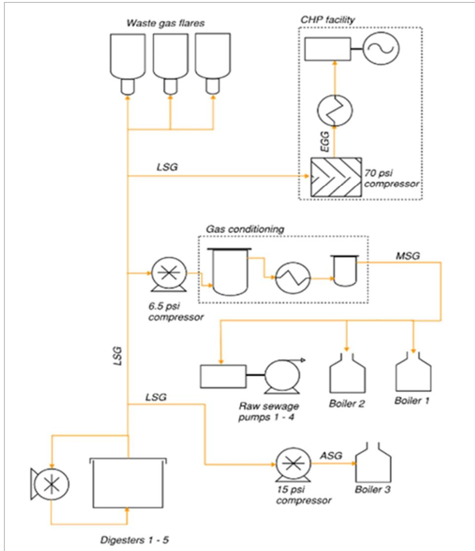
Figure 2-1. Existing Digester Gas Flow
