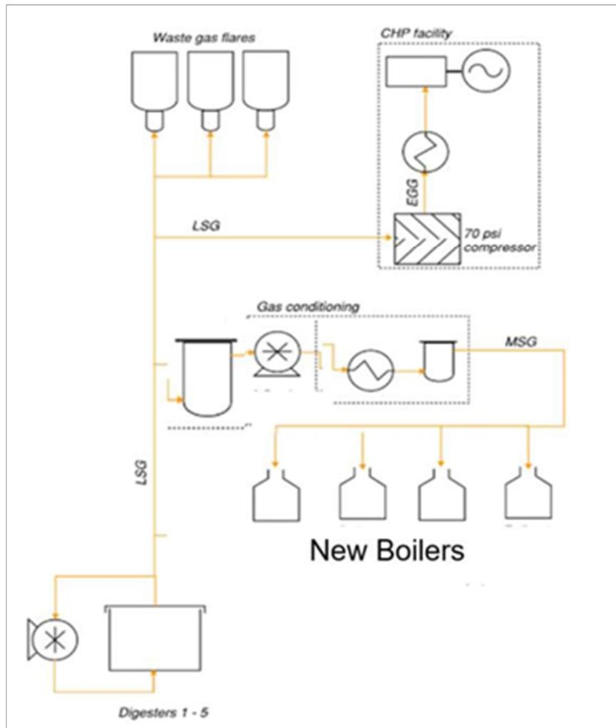
**Figure 2-2. Digester Gas Flow with Replacement Boilers**
